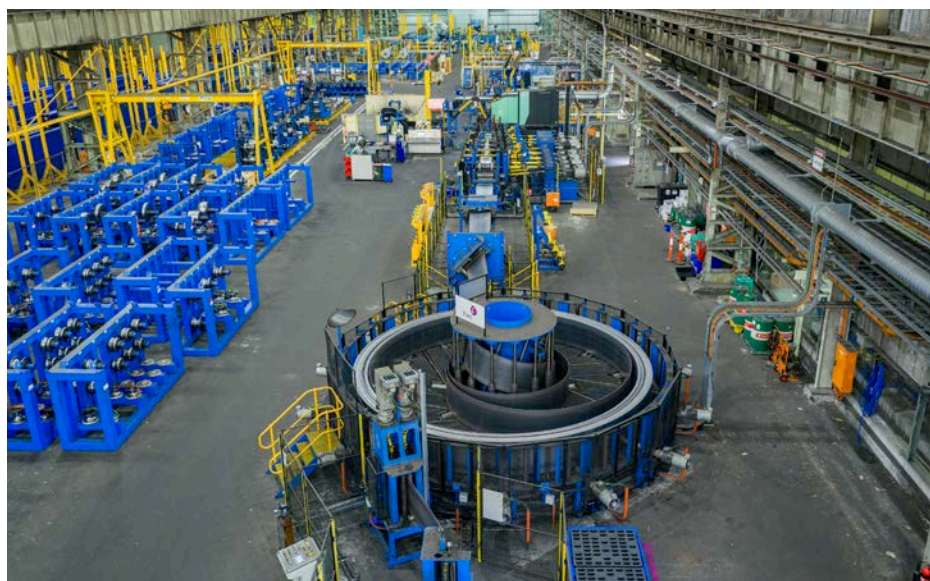
Fives automated OTO tube mill Orrcon Steel
