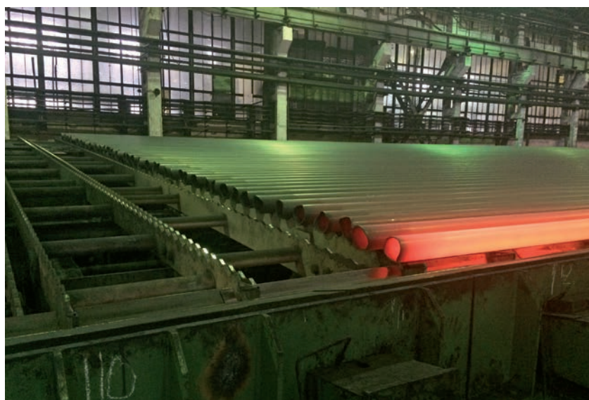
Seamless steel pipes on the cooling bed in the Tagmet PQF® mill.
