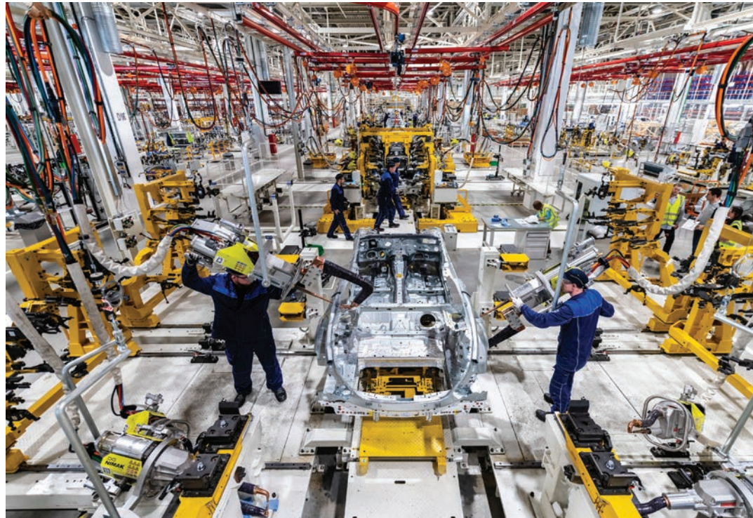
NIMAK manual welding guns in production at the new Mercedes-Benz assembly plant in Russia. Photo: Mercedes-Benz AG
